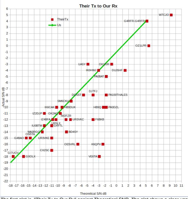
The first plot is "Their Tx to Our Rx" against Theoretical SNR. The plot shows a clear upper bound on the received SNR, and suggests that the maximum value of EIRPs of other stations are reasonably accurate.
