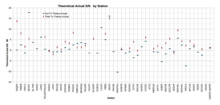
The third plot is "Theoretical SNR - Actual SNR for each direction by station". This is the same data as before, plotted by station (in order of date worked, left to right). Most stations seem to be around the +2dB level, and so maybe the theoretical SNR is a bit high.
